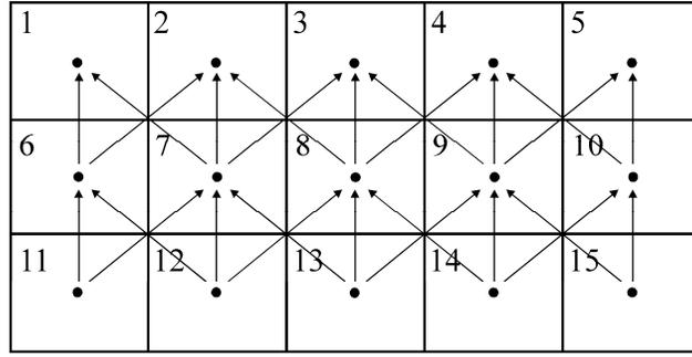
Fig. 1. Directed graph representing two-dimensional vertical ore body model
