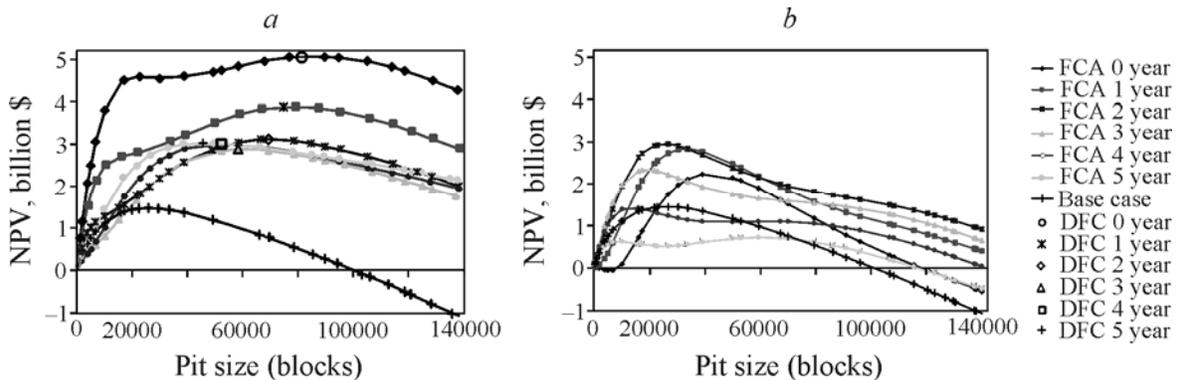
Fig. 3. Pit size versus NPV: FCA — floating cone algorithm; DFC — direct NPV FCA
